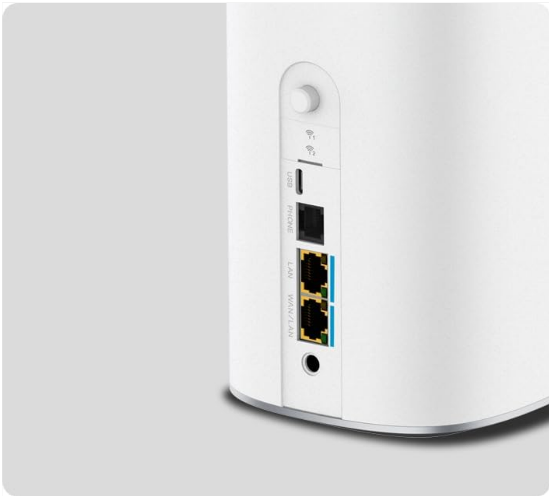
Figure 2: Rear panel of ZTE G5 Ultra MC8512 router. This image displays the rear panel of the ZTE G5 Ultra MC8512 router, detailing the various ports including USB, Phone, LAN, and WAN/LAN connections.
