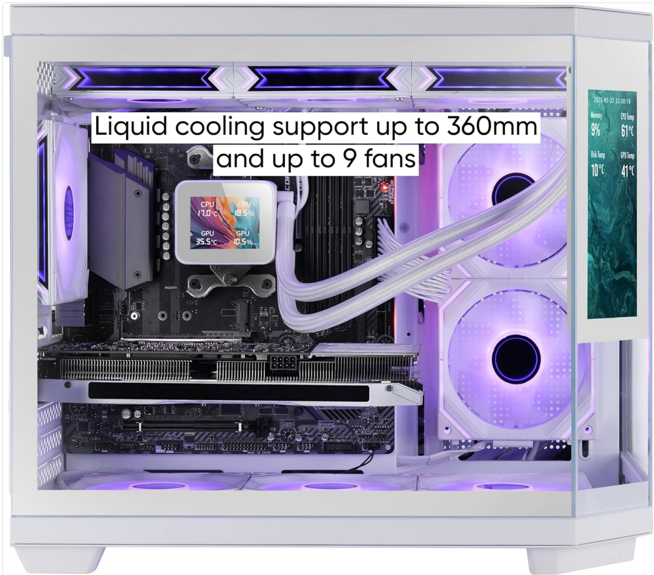
Figure 3: Example of liquid cooling installation within the MC-3TCORELCDM case, supporting up to 360mm radiators and multiple fans.
