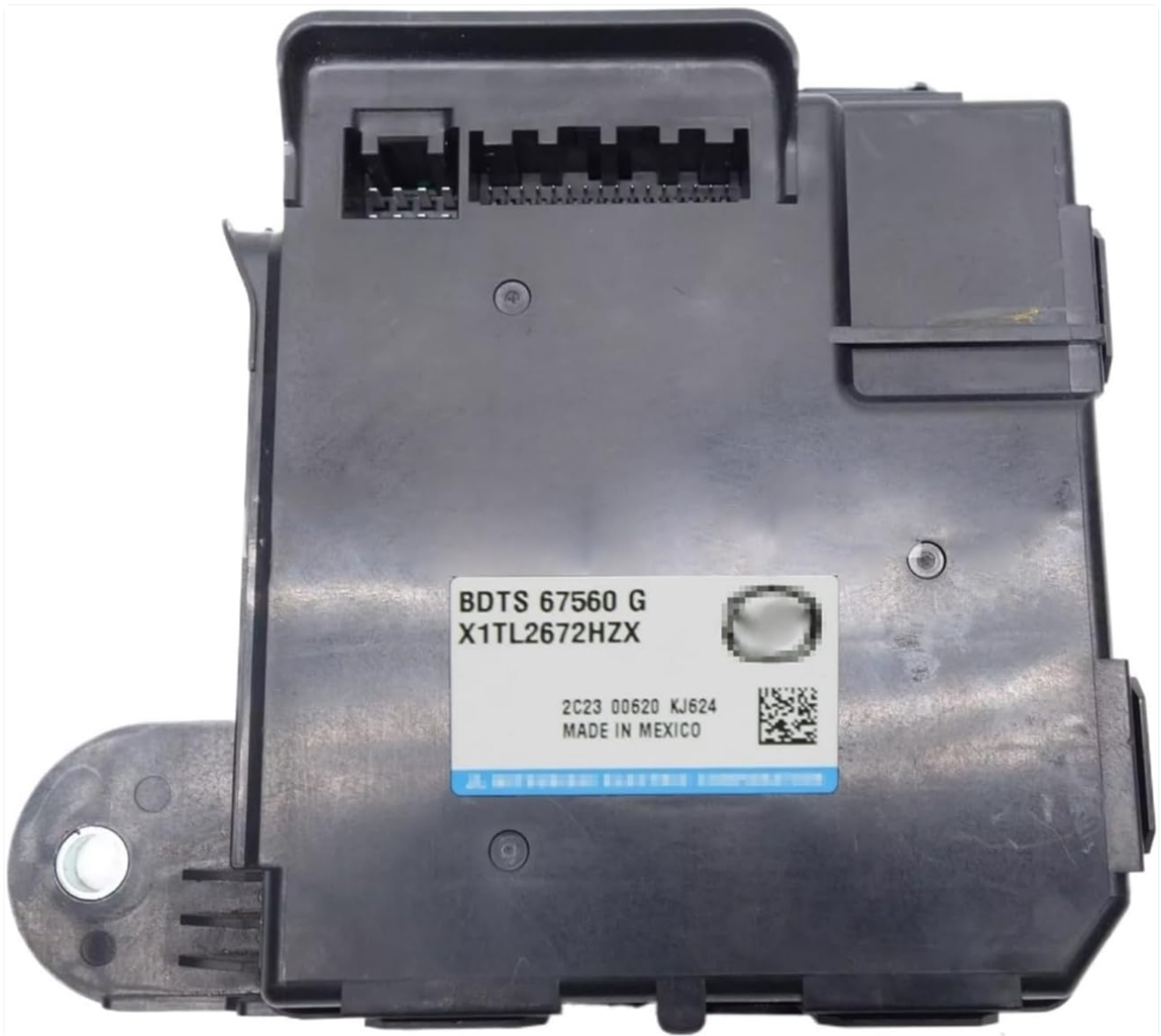
Image 1.1: Top view of the PJFJFP BCM Control Module Unit BDT67560G, showing the main label with part number and connectors.
