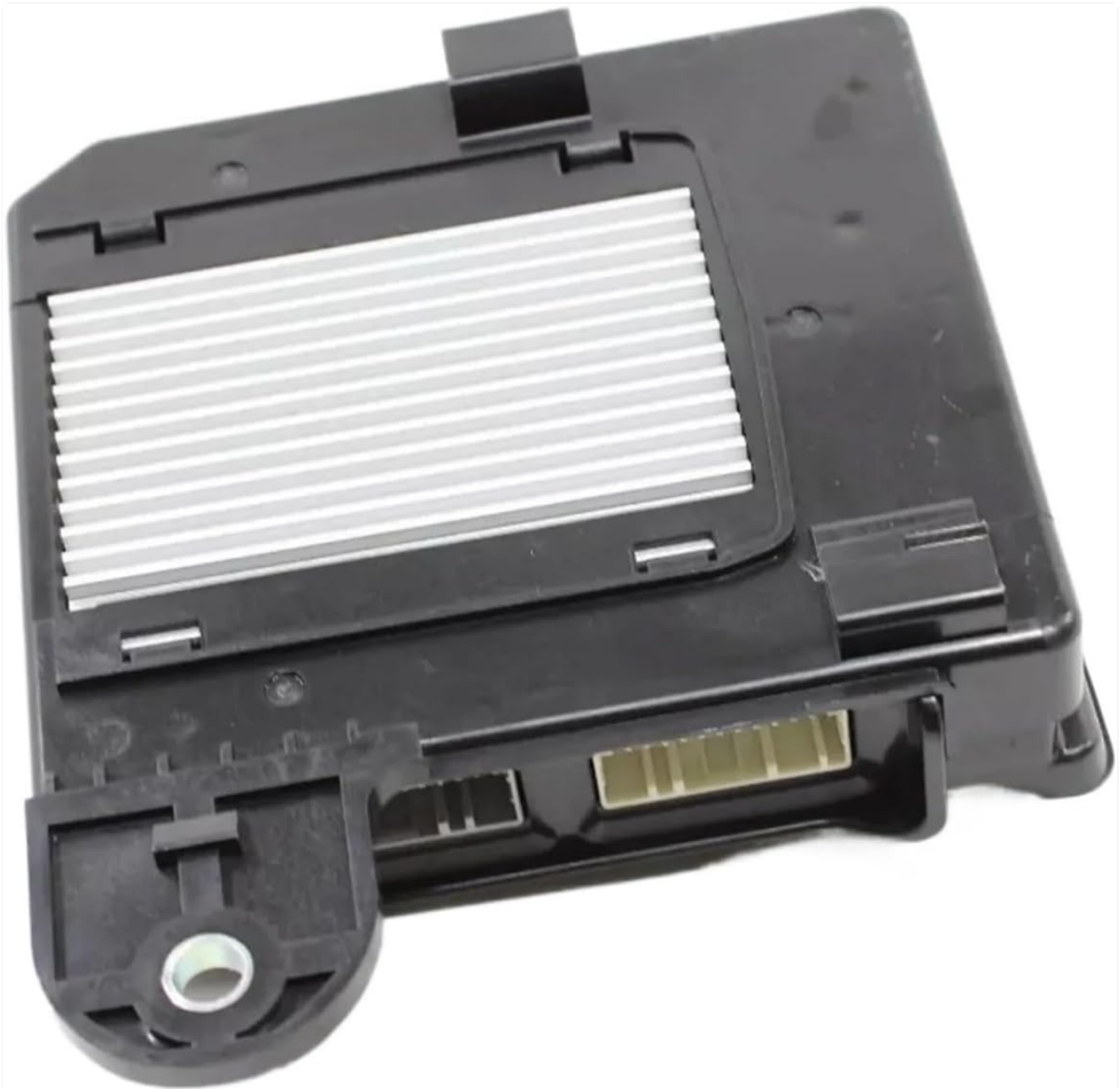
Image 4.2: Bottom view of the BCM unit, revealing the heatsink for thermal management.
