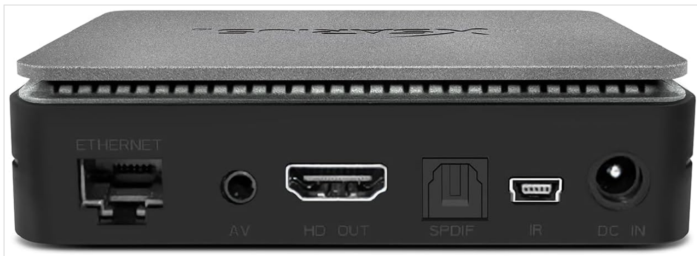
Figure 2: Rear panel of the Xsarius Sniper X2, illustrating the various connectivity ports.
