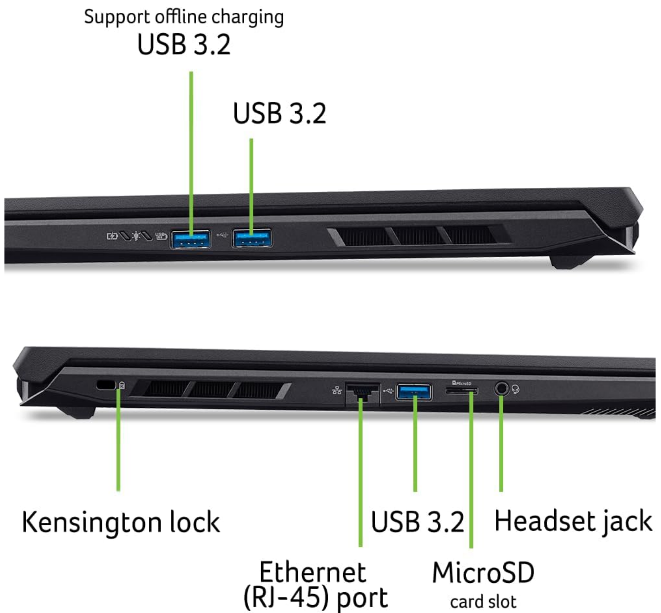
Figure 5: Left side of the laptop showing USB 3.2 ports, Kensington lock, Ethernet (RJ-45) port, MicroSD card slot, and Headset jack.
