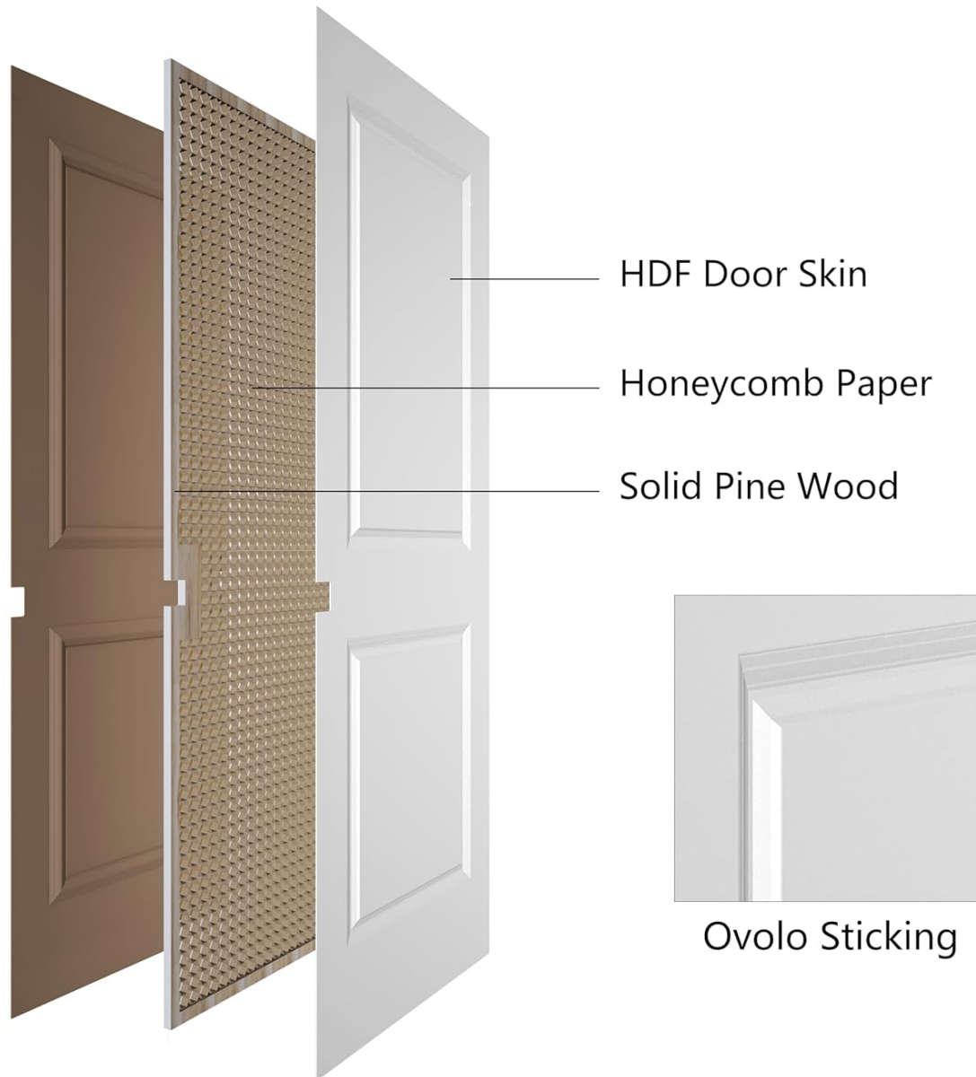
Image 3.2: An exploded view illustrating the hollow core construction of the door, showing the HDF door skin, honeycomb paper core, and solid pine wood frame, along with an Ovolo sticking detail.
