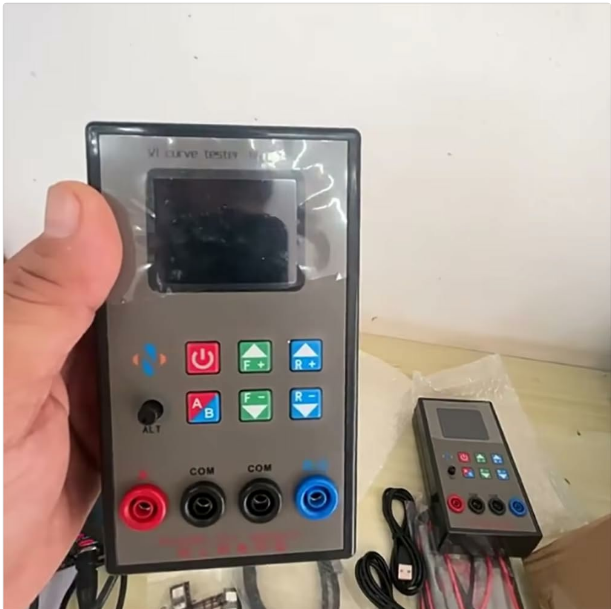
Figure 4.1: Front view of the device, showing the TFT screen, control buttons, and input ports.
