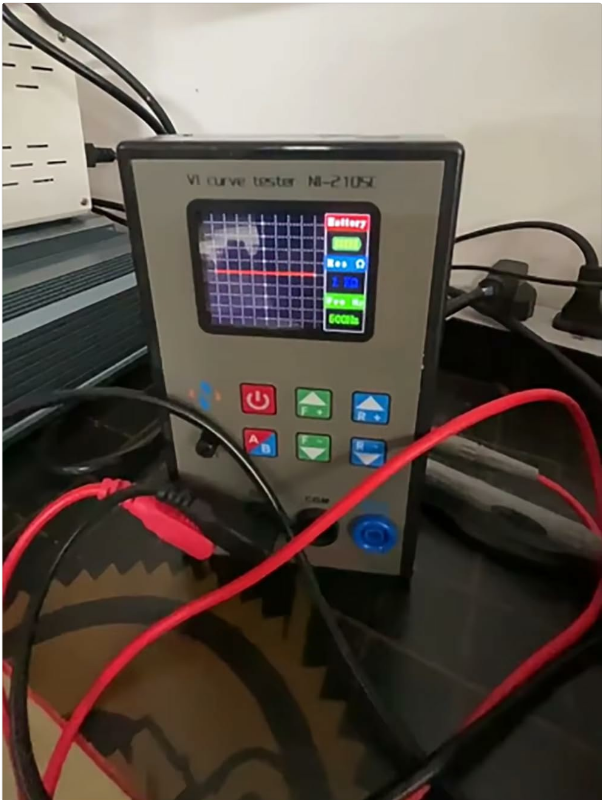
Figure 6.1: The VI Curve Tester in operation, connected to a circuit board for component analysis.
