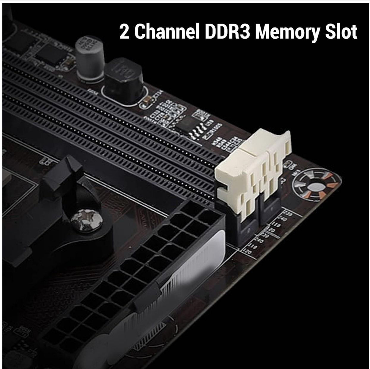
Figure 4.3: Close-up of the two DDR3 memory slots on the A78SD3 motherboard, indicating where RAM modules are to be installed.
