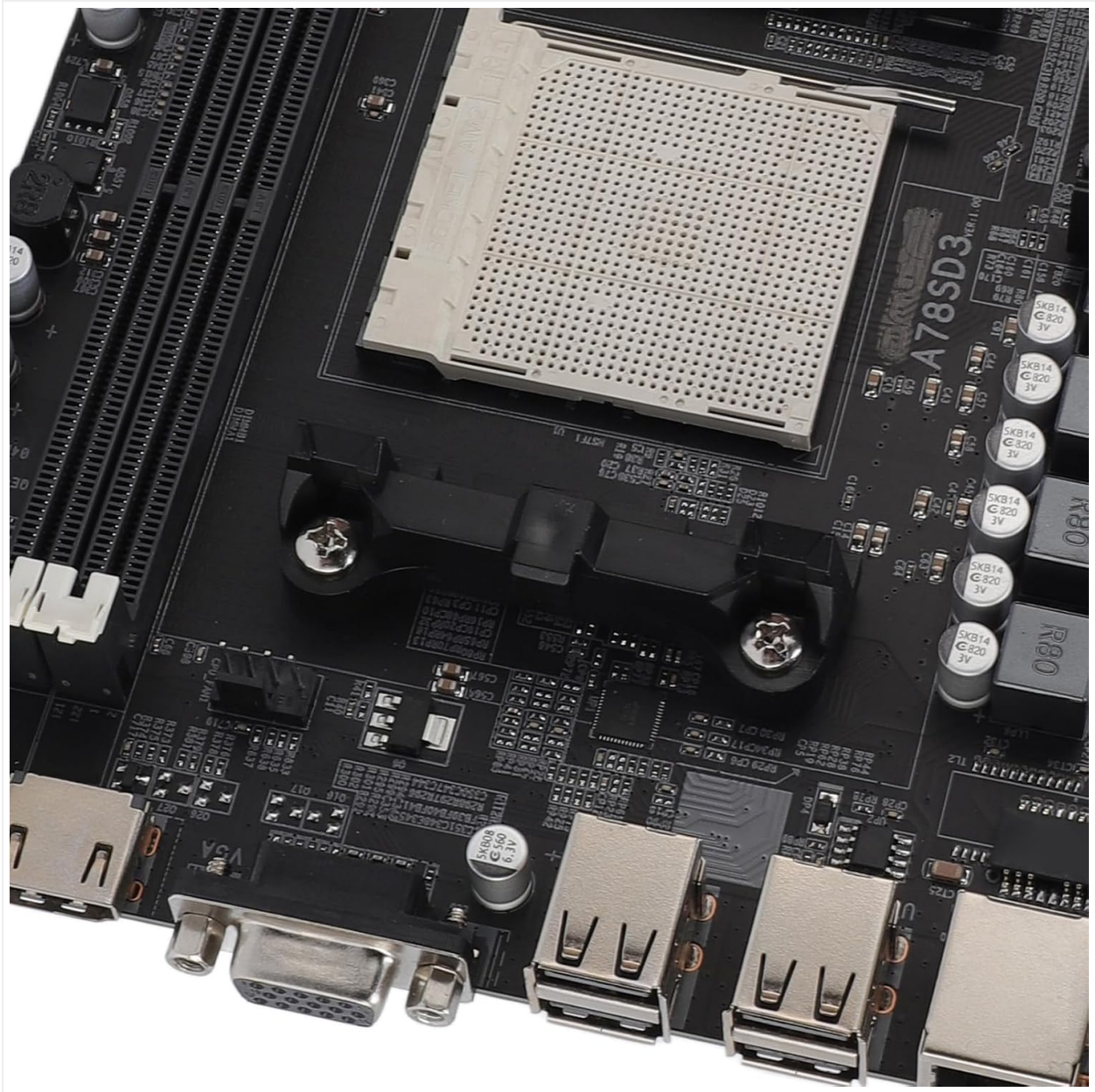
Figure 4.2: Close-up of the AM3 CPU socket on the A78SD3 motherboard, ready for processor installation.
