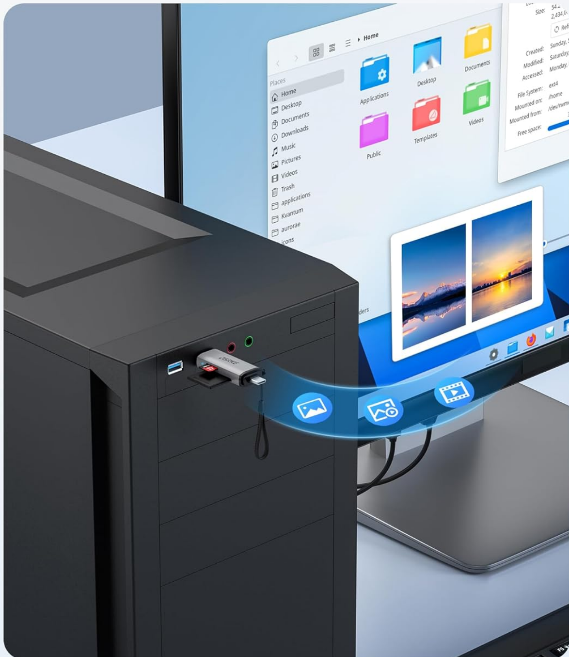
Image 2.1: The DSRKE card reader connected to a desktop computer, demonstrating its USB-A and USB-C dual port functionality.
