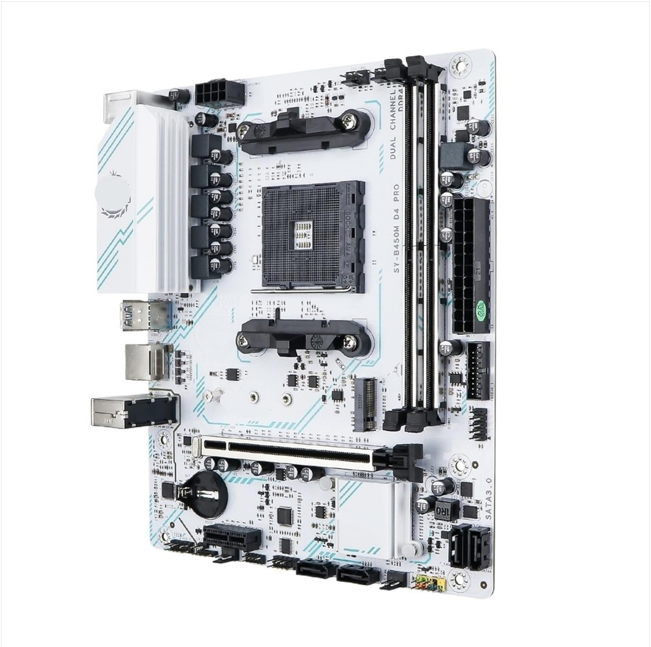
Figure 2: Angled view of the SOYO B450M motherboard. This perspective highlights the various I/O ports on the left, including USB, HDMI, and audio jacks, as well as the PCIe slots for graphics cards and other expansion cards.
