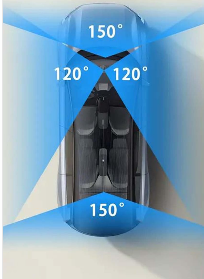
Figure 2.2.2: Illustration of the 360° total protection provided by the four cameras, showing the field of view for each.
