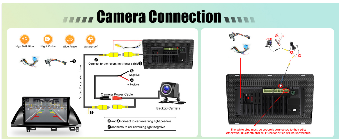
Image: A detailed wiring diagram showing how to connect the backup camera, including video and power connections to the head unit and vehicle's reverse lights.
