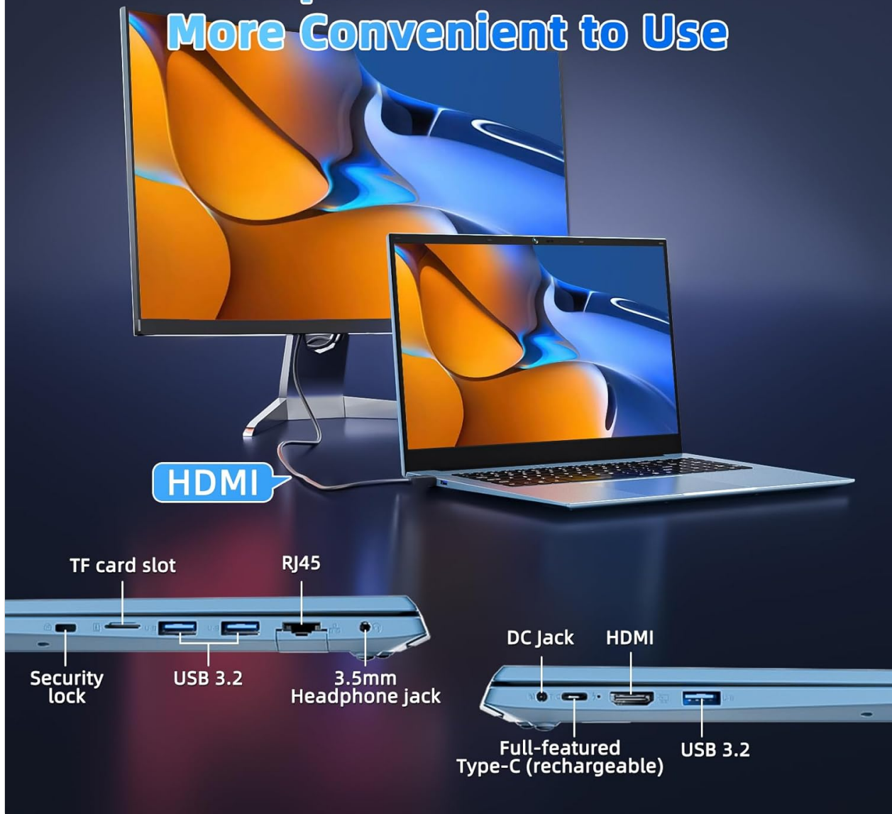
Image 6.1: An illustration detailing the various ports available on the SGIN S15 laptop, including HDMI, Type-C, USB 3.2, 3.5mm audio jack, TF card slot, and security lock.
