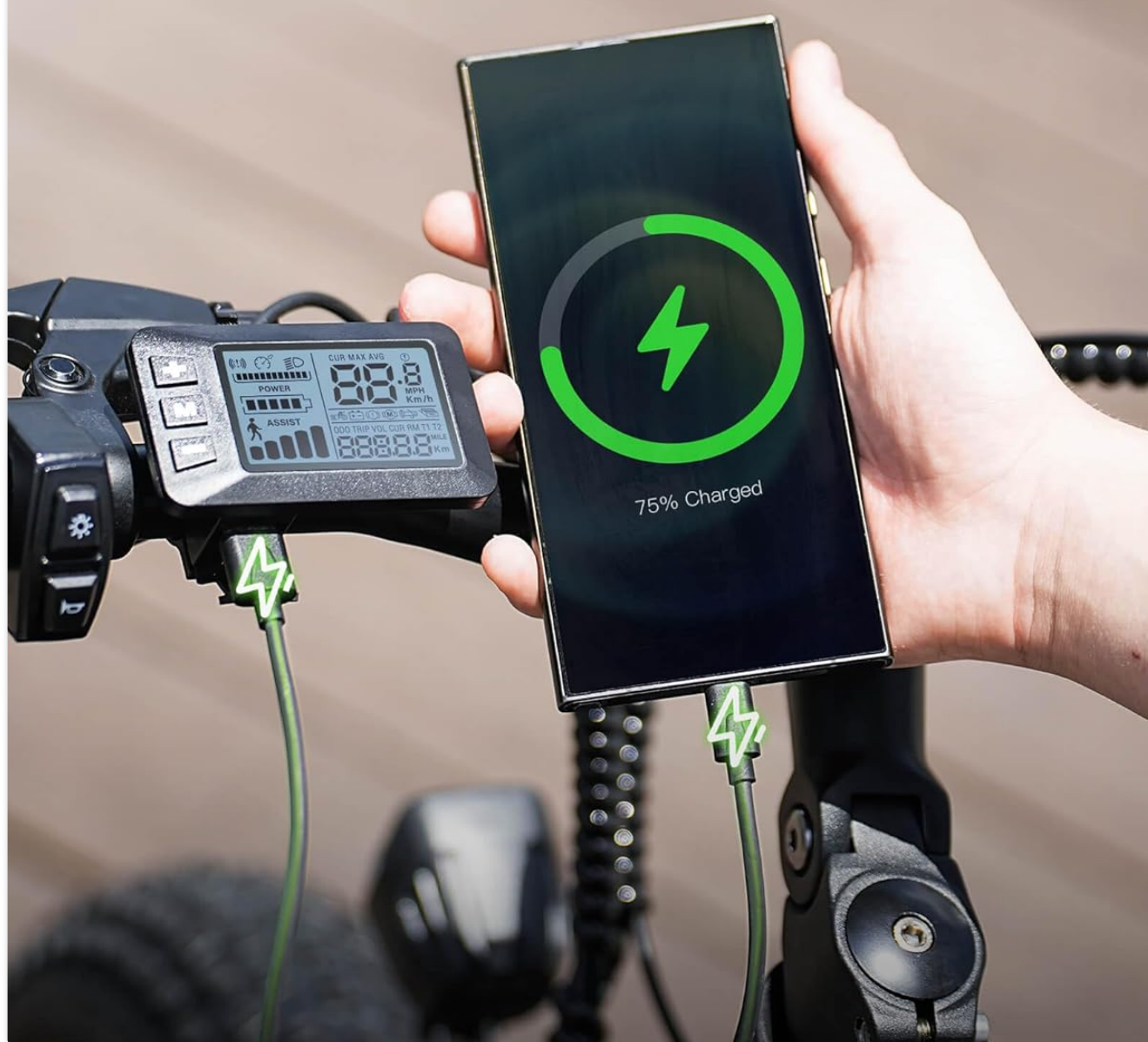
Image 4.2: A hand plugging a USB cable into the charging port located near the display on the handlebar.
