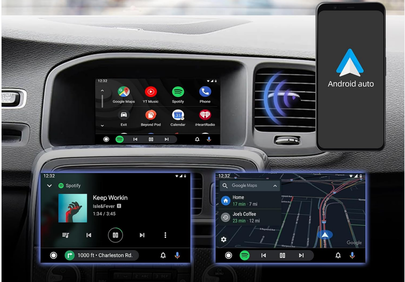
Image 5.3: Wireless Android Auto interface displayed on the vehicle's screen, showing music and navigation applications.
