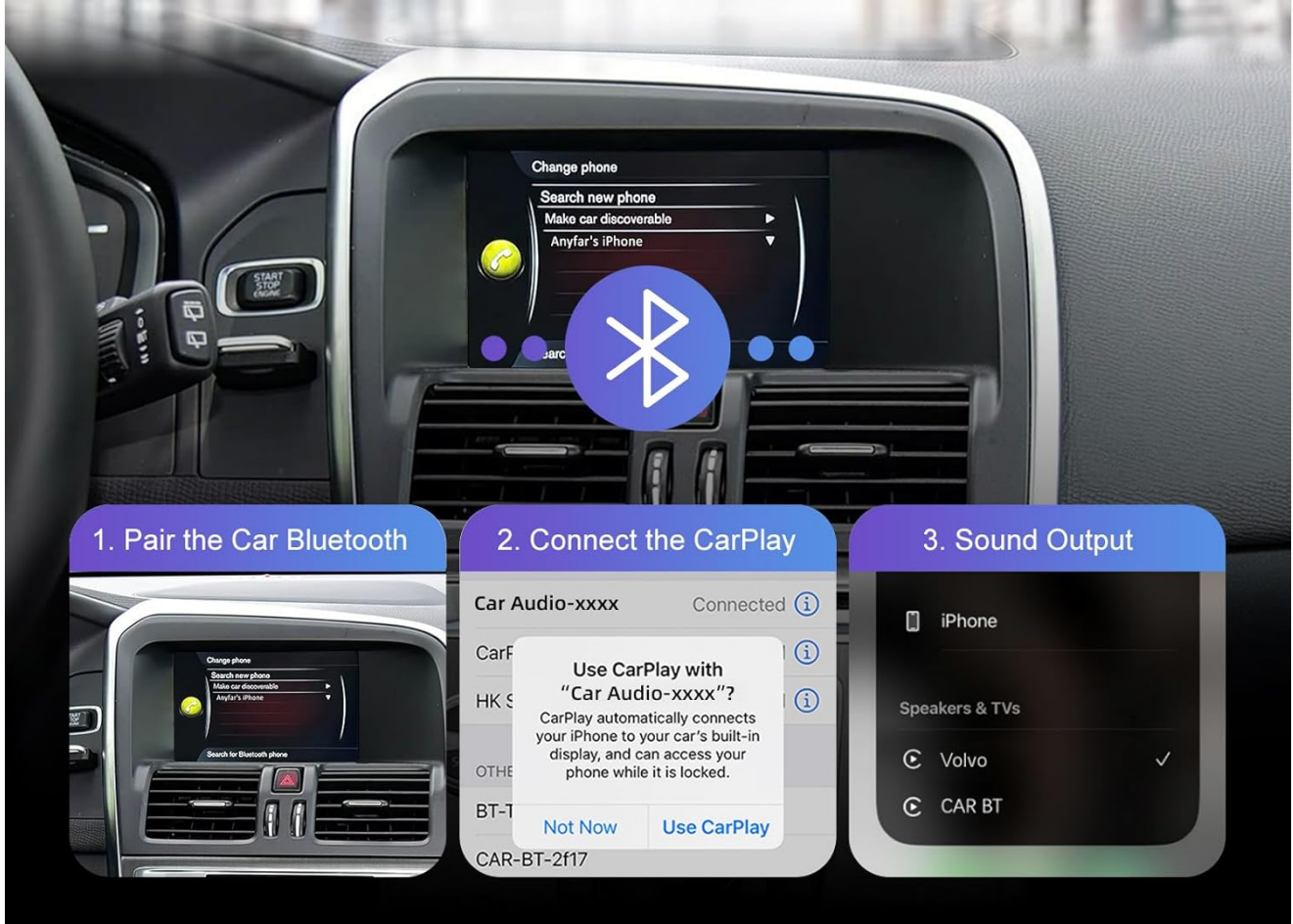
Image 5.5: Step-by-step guide for pairing your phone's Bluetooth and connecting to the CarPlay system for audio output.
