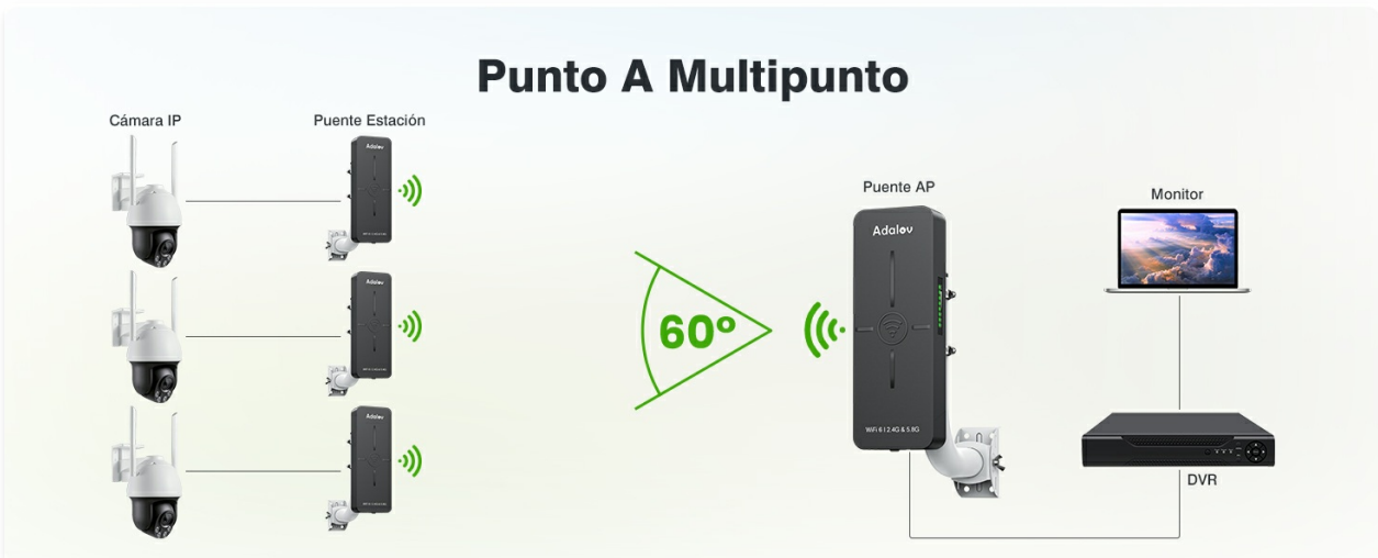
Figure 4.2: Point-to-Multipoint network configuration.
