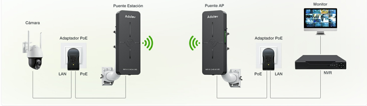
Figure 4.5: P2P application for security camera systems.
