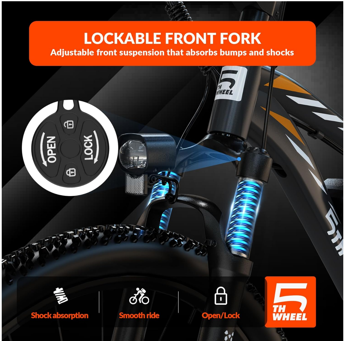
Image: Detail of the lockable front suspension fork, showing the adjustment dial for different riding conditions.
