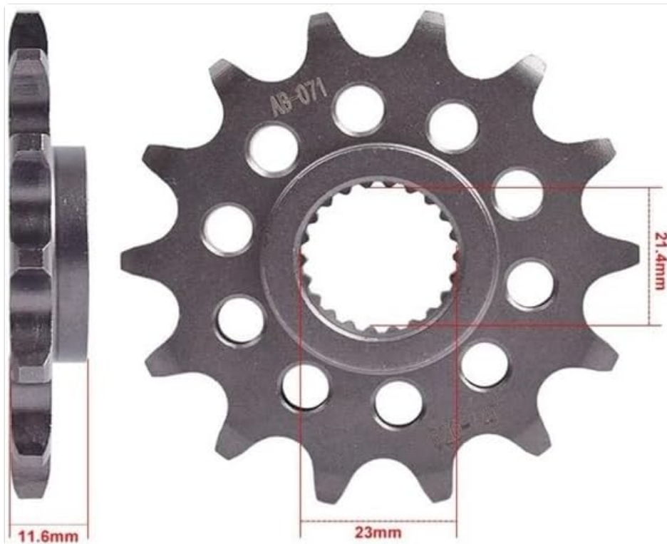
Image 2: Detailed view of the Generic Motorcycle 520 14T Front Sprocket with key dimensions. This image shows the sprocket from the top and side, indicating measurements such as the 21.4mm installation size, 23mm width, and 11.6mm total thickness.
