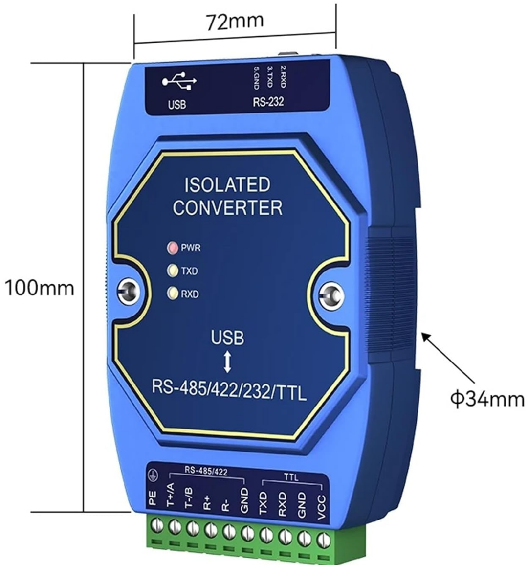
Figure 1: E810-U15 Industrial Converter with dimensions (100mm x 72mm x 34mm) and port labels for USB, RS-232, RS-485/422, and TTL.
