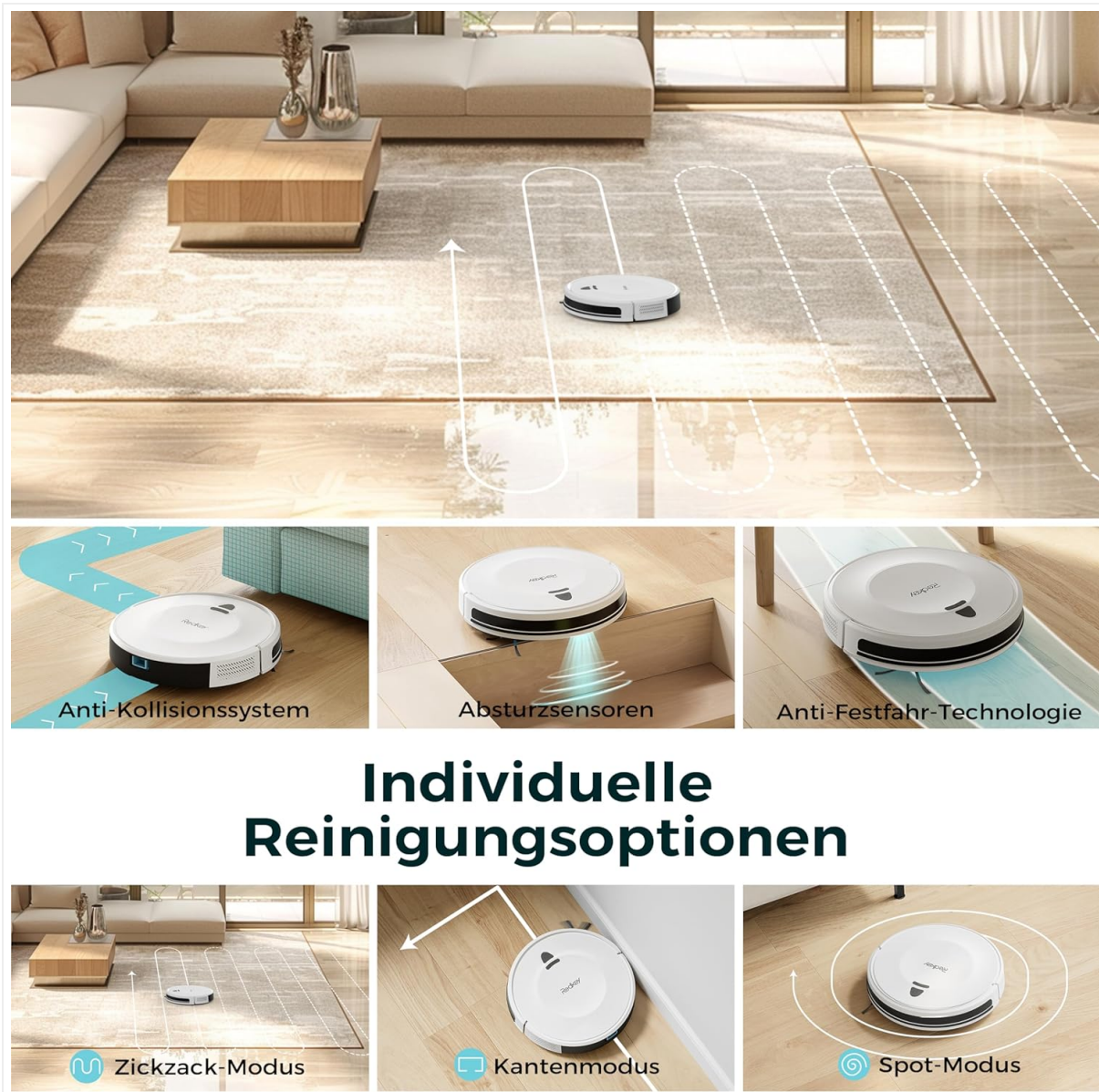
Figure 5.1: Illustration of the Redkey E6's intelligent navigation (zigzag mode) and protective sensors, including anti-collision, anti-fall, and anti-stuck technologies, along with various cleaning options like Edge Mode and Spot Mode.
