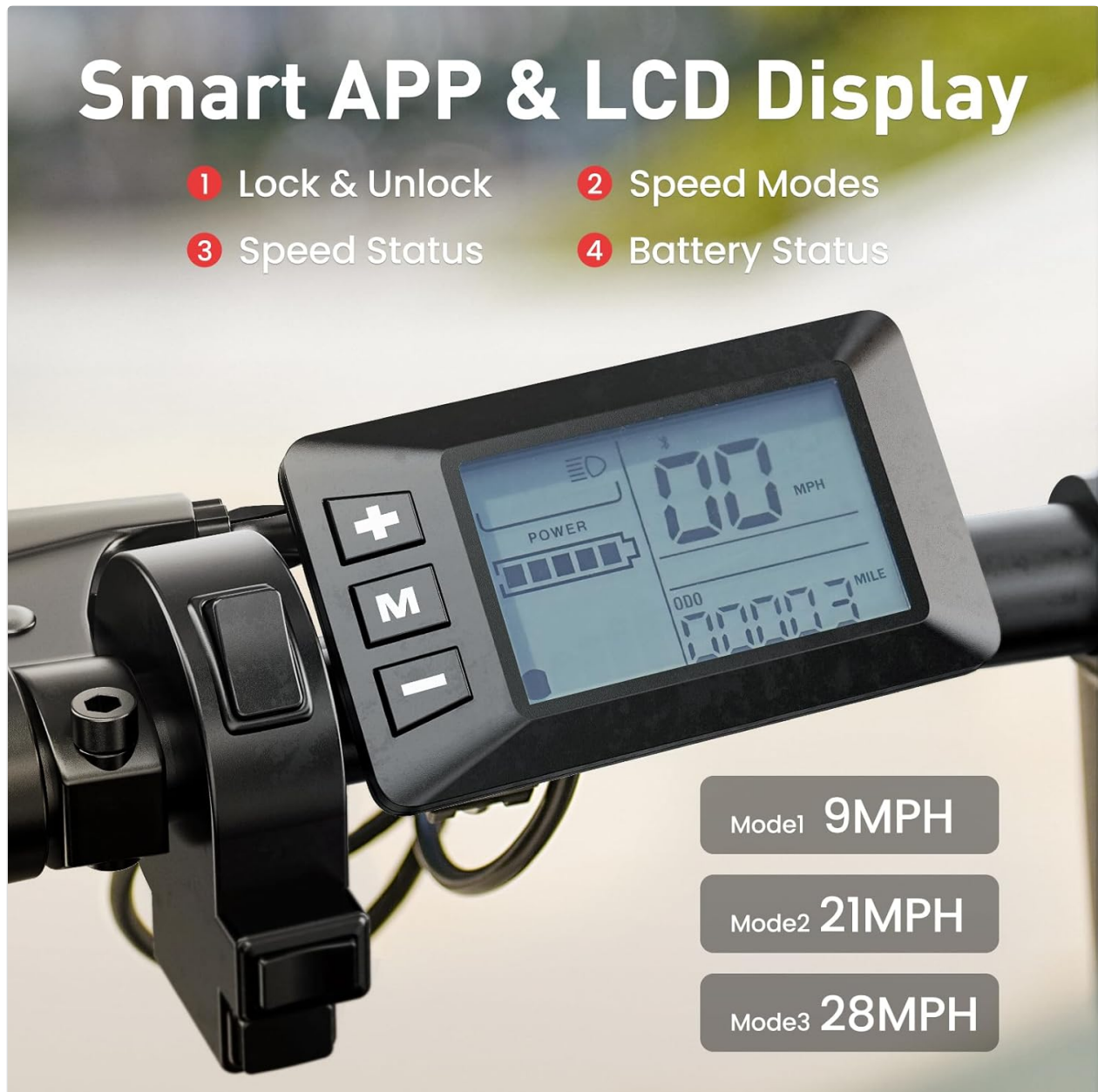
Image 5.1: The LCD display of the iScooter F7, illustrating the speed modes (9, 21, 28 MPH) and battery status indicators.
