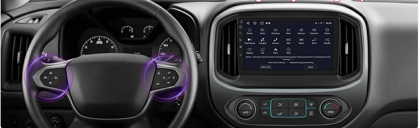
Image: A driver's view of the steering wheel with highlighted controls, demonstrating how the car stereo integrates with the vehicle's steering wheel controls for safe operation.
