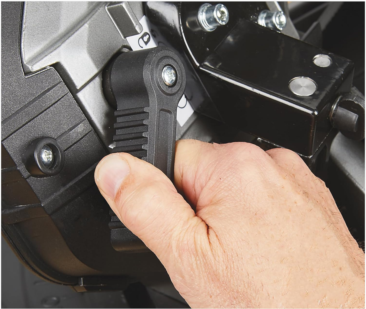
Figure 2.6: The quick-release lever for detaching the saw from its benchtop base.
