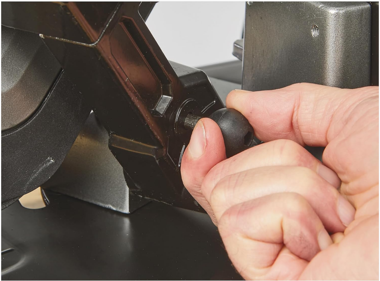
Figure 2.7: The tool-less knob for adjusting the blade guide, ensuring proper blade alignment.
