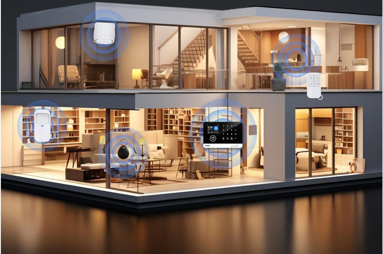
Figure 4.1: Recommended placement of the alarm host and various sensors within a home environment. The diagram illustrates the alarm hub, PIR motion sensor, door & window sensor, wireless strobe siren, gas detector, WiFi doorbell, outdoor camera, and smoke detector in different areas of a house.
