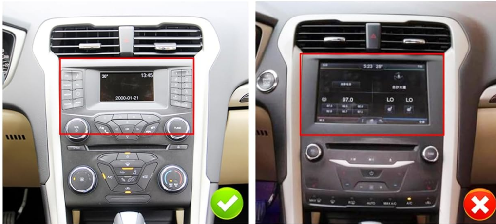
Image 2.1: Visual guide for checking vehicle center control consistency before installation. Ensure your vehicle's original setup matches the 'Before Installation' image for proper fitment.
