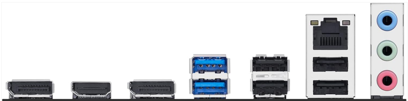
Image: Close-up view of the rear I/O panel, showing HDMI, USB 3.2 Gen 1, USB 2.0, 1Gb LAN, and audio ports.
