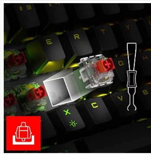
Image: An illustration demonstrating the process of removing a mechanical switch from the keyboard using a switch puller.
