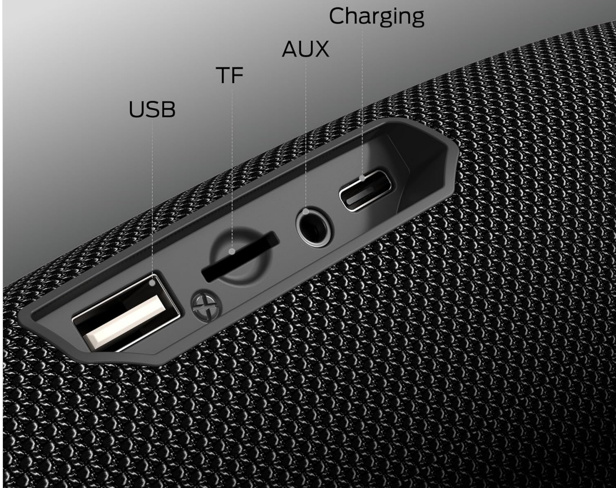
Figure 4.3: Multi-connectivity ports (USB, TF, AUX, Charging).
