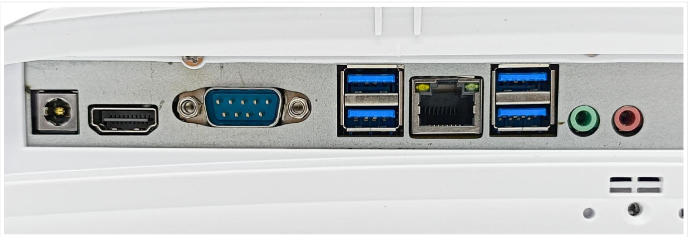
Image 3.3: Rear ports of the AIO-2755C, including HDMI, USB 3.0, Ethernet, and audio jacks.
