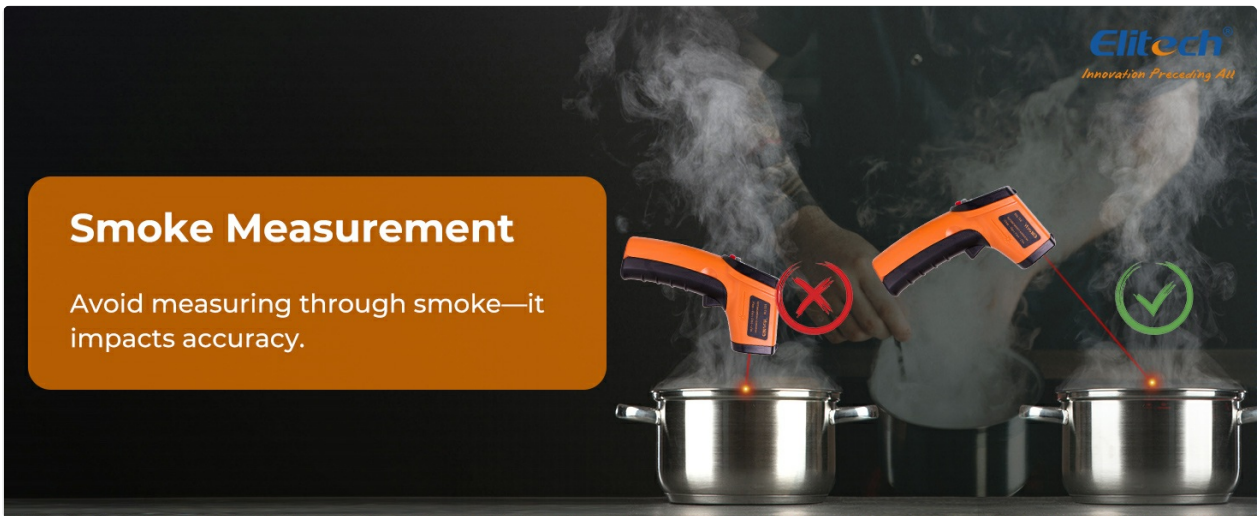
Figure 8: Smoke Measurement Accuracy
