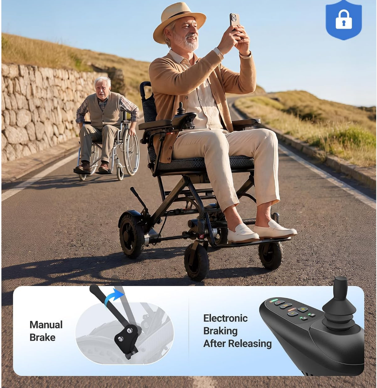
Figure 3.2: The wheelchair features both an automatic electronic braking system that activates upon joystick release and a manual brake for secure parking.
