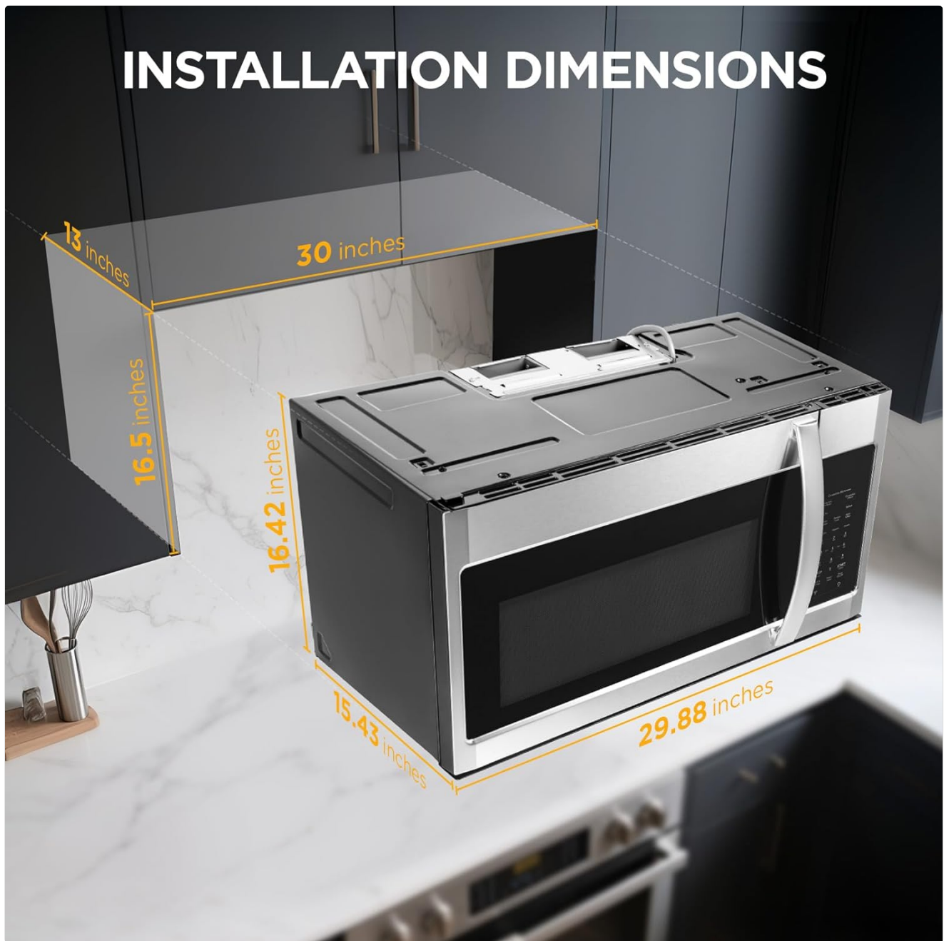
Figure 3.1: Installation dimensions. The microwave measures 29.88 inches (W) x 16.42 inches (H) x 15.43 inches (D). Ensure cabinet depth is at least 13 inches and height clearance is sufficient.
