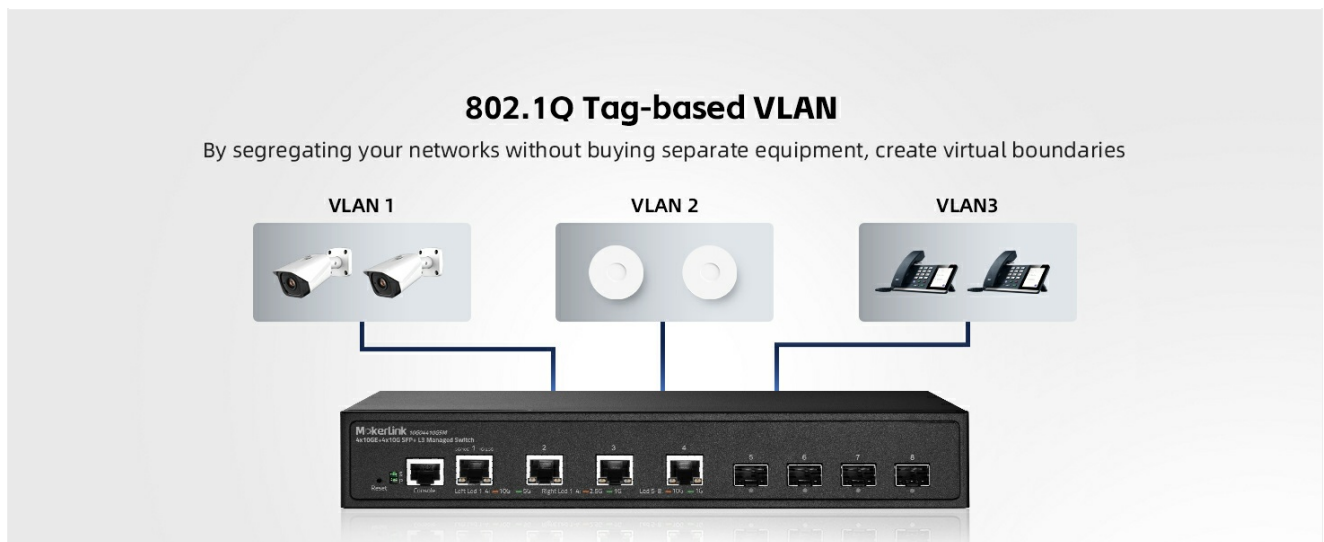
Figure 6.1: Example of 802.1Q Tag-based VLANs segregating network traffic for different devices like cameras, servers, and IP phones.
