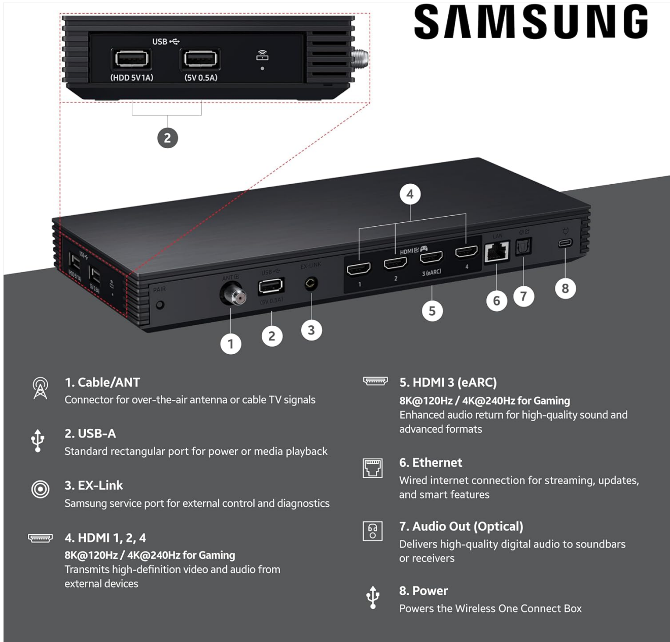
Figure 3: Detailed diagram of the Wireless One Connect Box ports.
