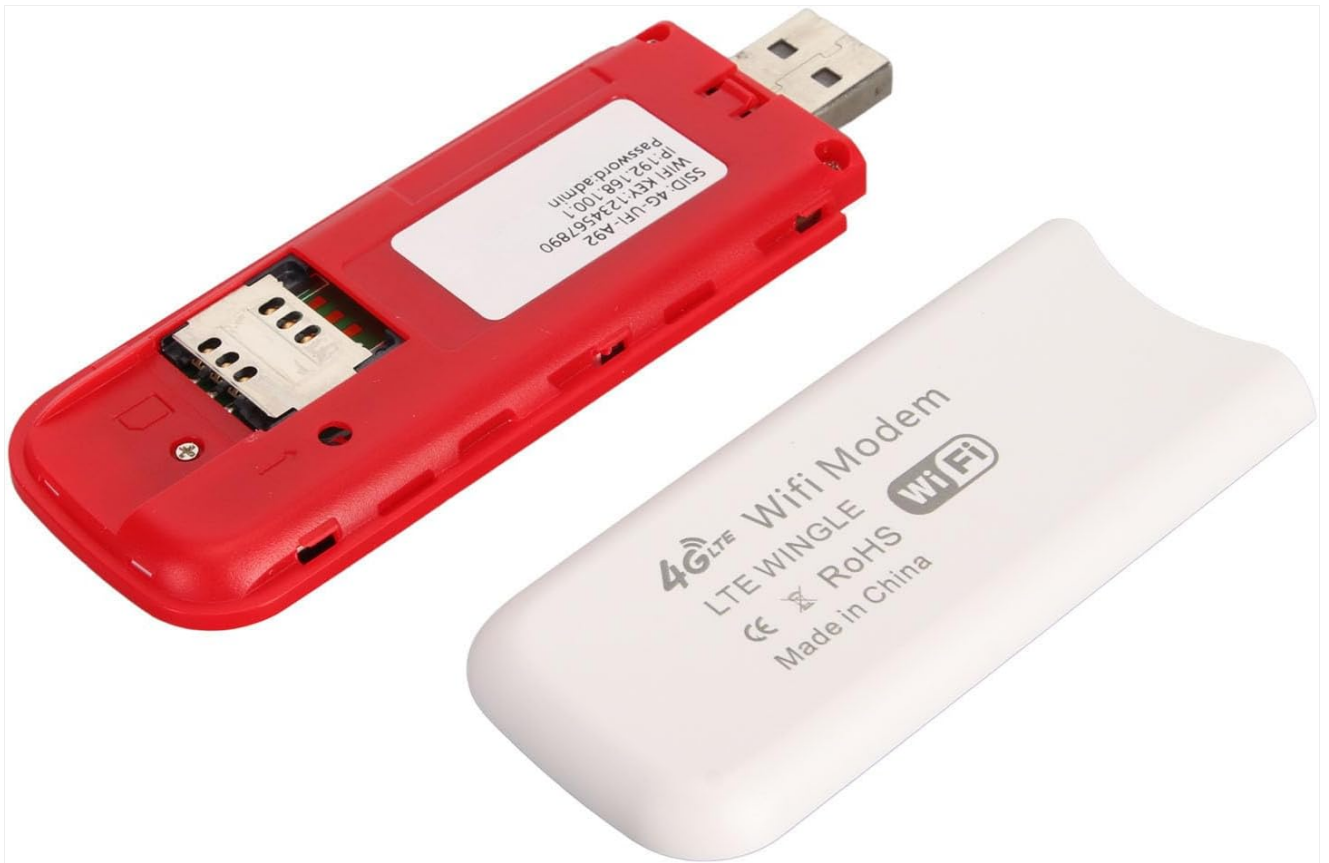
Image showing the SIM card slot after removing the back cover.
