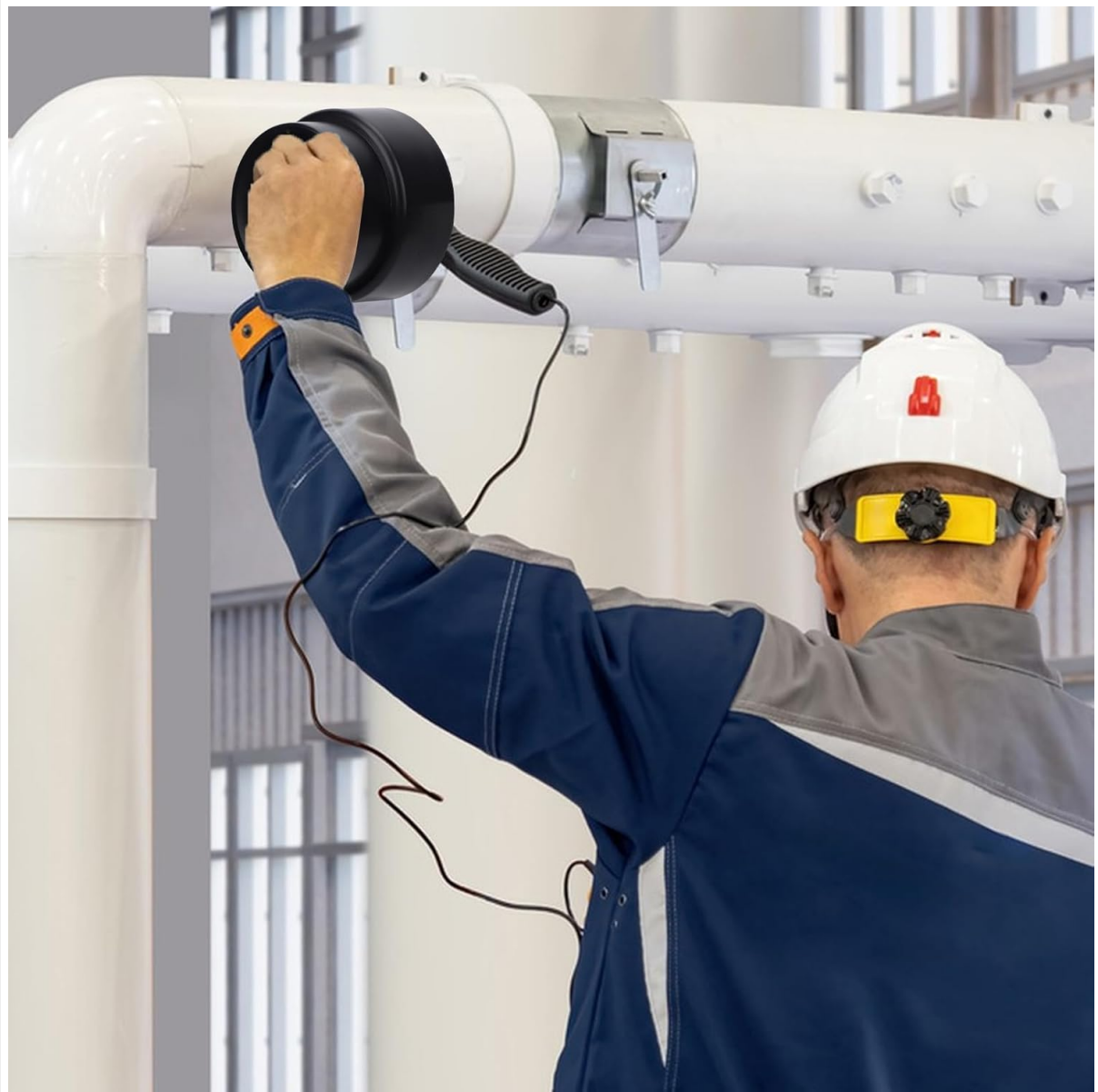
Image: A technician using the GOWENIC detector to listen for leaks on an overhead pipe.
