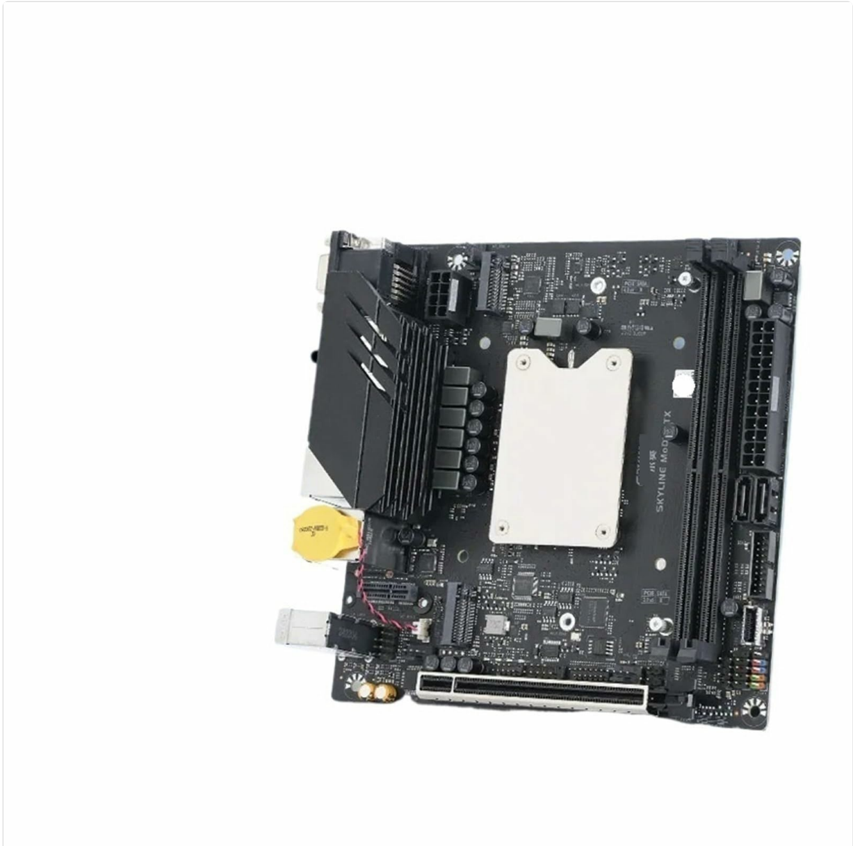
Image 1: ERYING ITX Gaming Motherboard. This image displays the compact ITX form factor motherboard, highlighting the CPU heatsink mounting area, DDR4 RAM slots, PCIe 4.0 slot, M.2 slot, and various rear I/O ports including USB, audio, and video outputs. The integrated CPU is located under the central heatsink mounting bracket.
