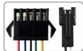
Figure 3: Product Plugs. This image shows the GD02 display, its integrated cable, and a close-up of the 5-pin SM connector, highlighting the connection points.
