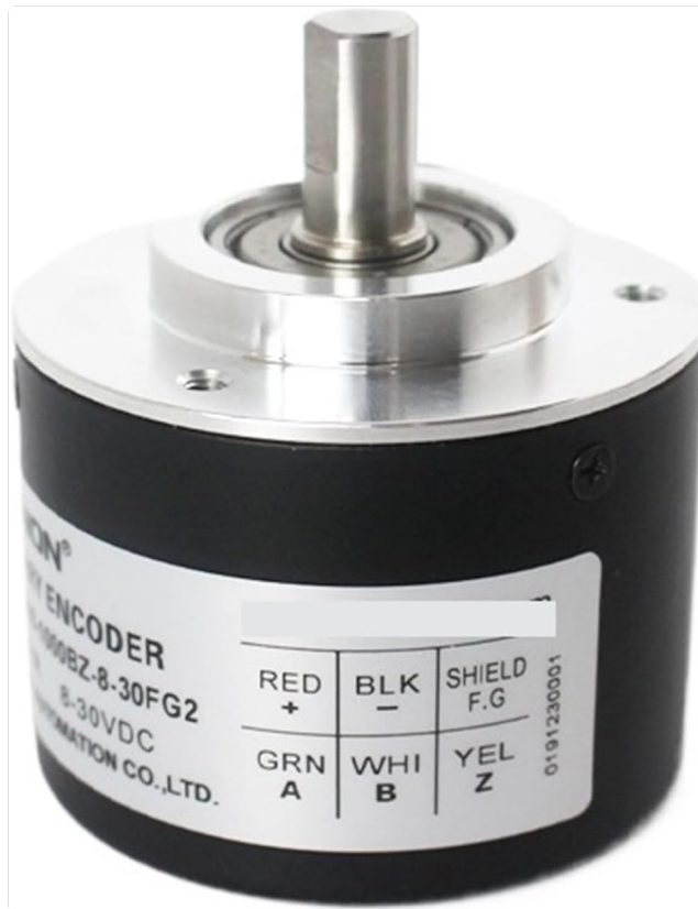
Image 1: F7X3K0Z CSP50/8-1000BZ-8-30FE Encoder showing its main body, shaft, and a label with wiring color codes and corresponding functions. The label indicates connections for power, ground, shield, and output signals A, B, and Z.
