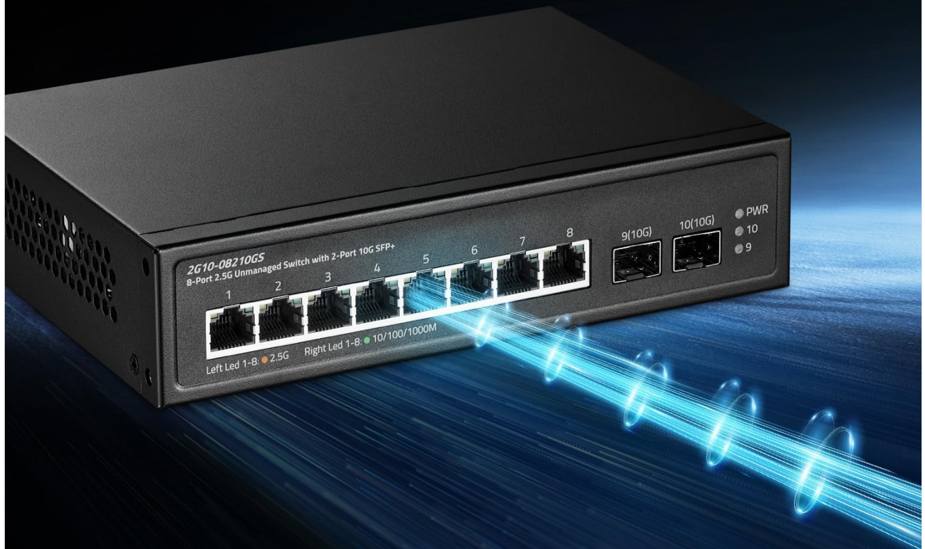
Image 1.1: Binardat 10-Port 2.5G Unmanaged Ethernet Switch, highlighting 8x2.5G ports and 2x10G SFP+ ports.
