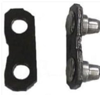
Image: A single preset link and a tie strap from the FACULX repair kit, illustrating the two main components.
