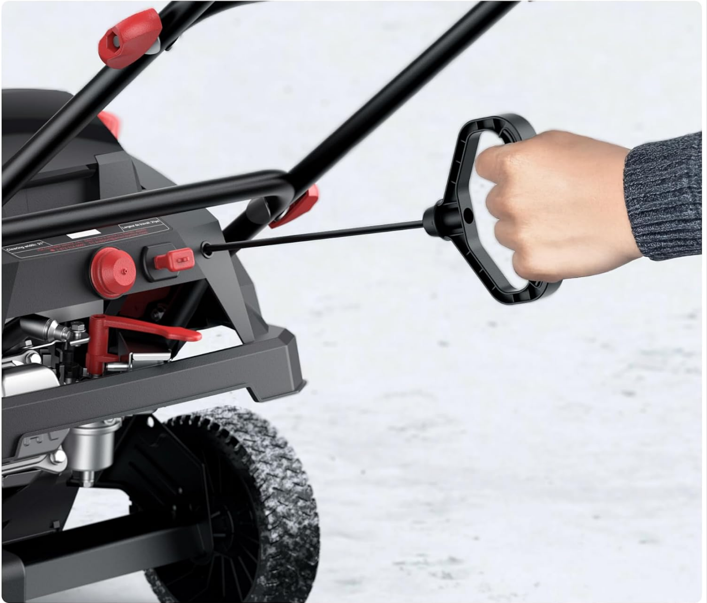
Figure 2: The recoil start handle for manual engine ignition.
