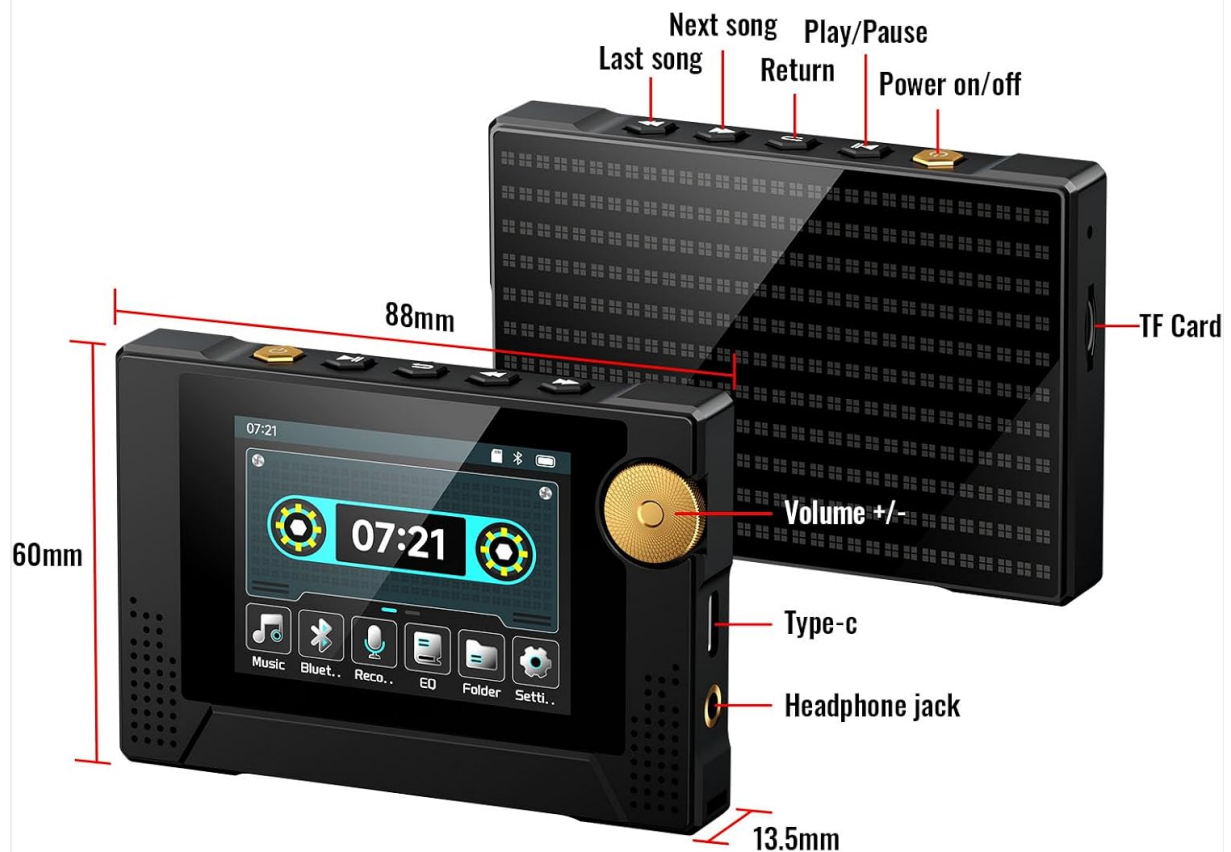
Image: Detailed diagram of the Phinistec F18 MP3 Player, highlighting the power button, volume scroll wheel, navigation buttons, Type-C port, headphone jack, and TF (SD) card slot, along with its dimensions.
