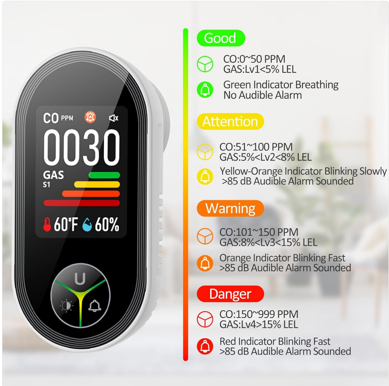
Image: The detector's screen is shown with a detailed legend explaining the different CO (Carbon Monoxide) and GAS (Combustible Gas) levels. It categorizes levels into "Good" (green indicator, no audible alarm), "Attention" (yellow-orange indicator blinking slowly, >85 dB audible alarm), "Warning" (orange indicator blinking fast, >85 dB audible alarm), and "Danger" (red indicator blinking fast, >85 dB audible alarm), providing clear visual cues for safety.
