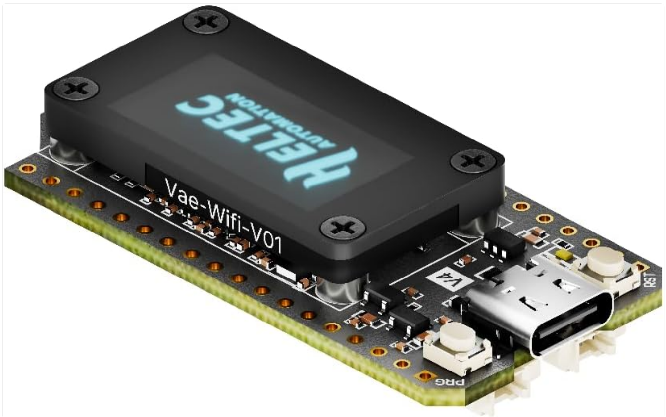
Figure 4: Close-up view of the Heltec WiFi LoRa 32 V4 Development Board, highlighting the integrated OLED display and USB-C port.
