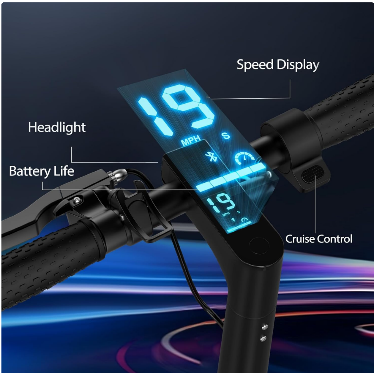
Image 6.1: LED Display showing Speed, Headlight, Battery Life, and Cruise Control.
