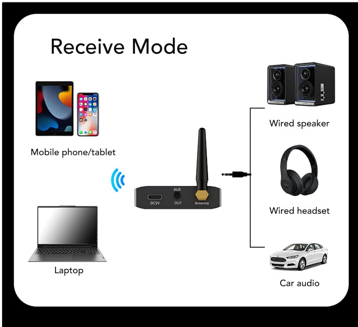
Image: A visual guide demonstrating how to set up the adapter in Receiver Mode, showing wireless connections from mobile devices or laptops to the adapter, and then wired connections to various audio output devices.
