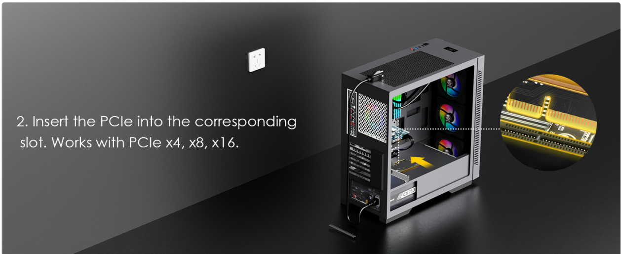
Image: Illustration of inserting the PCIe network card into an available slot on the motherboard.
