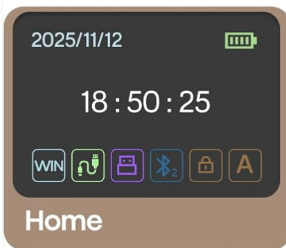
Image 3.2: The magnetically detachable mini screen displaying time, date, and various modes like DIY pictures/GIFs and Type-Writer Mode.
