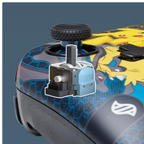
Image: Diagram showing the internal mechanism of a Hall Effect thumbstick.
